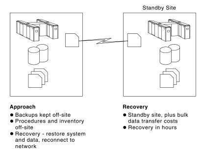
Figure 20. Disaster recovery tier 3: electronic vaulting
